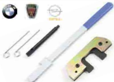
Para modelos BMW 318 TD/TDS, 325 TD/DS, 525 TD/TDS, 725 TD/TDS, Range Rover TD5/P38, 2.5D y, Opel Omega 2.5
